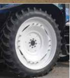
**The Heavy Duty Flange Rowcrop is unique to Stocks,** and is an extremely tough, good looking wheel suitable for 50 kph tractors. Rowcrop wheels are often subject to maximum loading, high road speeds and a hard ride due to higher tyre pressures. Stocks HDF wheels are designed to withstand the high loads imposed by large high speed tractors using front and rear mounted implements, and are manufactured to strict tolerances to ensure true running.
